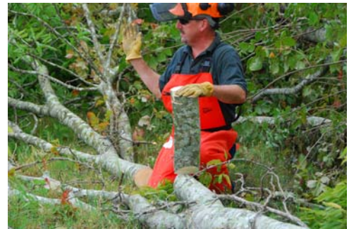
Dana Hinkley demonstrates a cutting technique to free a pinned logger. Use biodegradable bar & chain oil or vegetable oil. Mineral bar & chain oil will add infections to an already-injured person.
